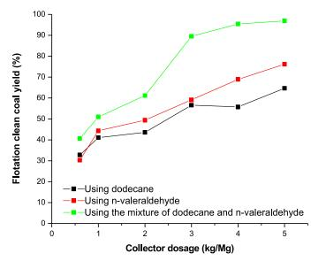
Fig. 5. Flotation results using different collectors
