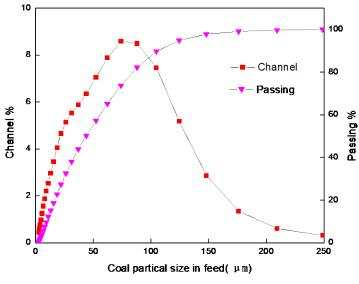
Fig. 2. Size distribution of coal sample
