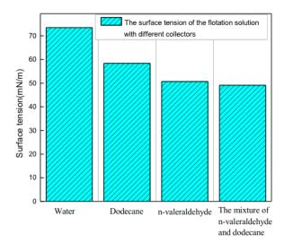
Fig. 9. The surface tension of the flotation solution with different collectors
